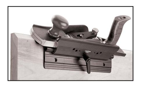
This plane fence does not limit you to right angles; it can be used to accurately and consistently plane any angle from 45° to 135°. It attaches to the plane body with a pair of locking knobs that can be positioned along a T-slot track to accommodate the differing plane sizes and geometries. It can be attached to either side of the plane (for right- or left-handed use).
