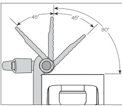
Figure 4: Setting the fence angle.
