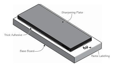
Figure 1: Plate attached to a base.
