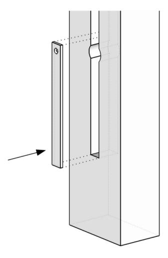
Install the bearing plates into the leg and the chop at the bottom of the mortises. They should slip into the mortise easily and rest on the bottom end of mortise and flatly on the back wall. Make sure you don't trap any wood shavings or chips behind the plate. They need to be flat to the mortise wall. Position the countersunk hole at the top, predrill, then drive the included wood screw to secure the plate.
